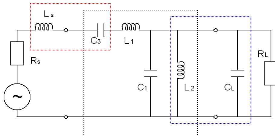
At resonance, the values of  $C_3$  and  $L_2$  are given as follows:
