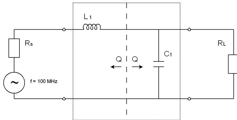
The quality factor has to remain the same on both sides of the network. We have a series circuit on the left and a shunt circuit on the right, so we can write:
